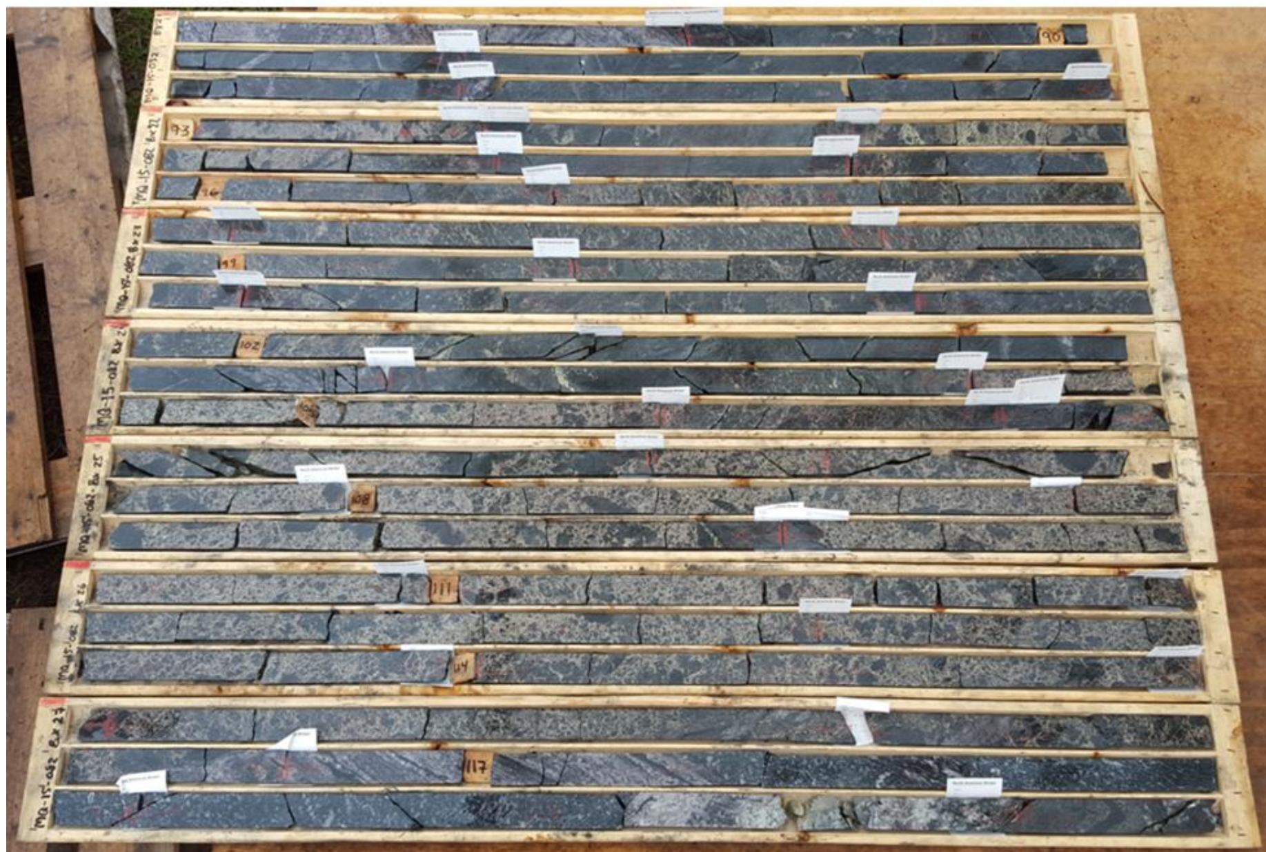
Figure 4: Intersection of mineralized drill core from hole MQ-15-082. Core is BTW size with a diameter of 41mm.
