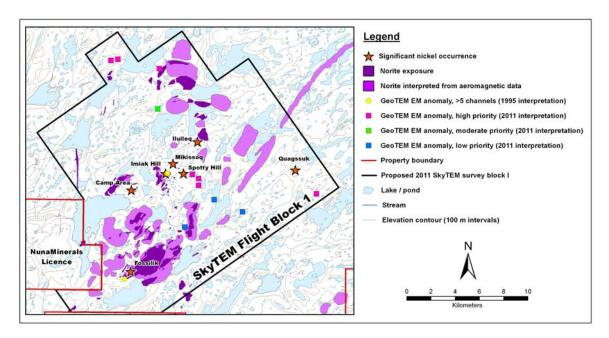
Figure 2: Map showing location of helicopter TEM survey block 1.
